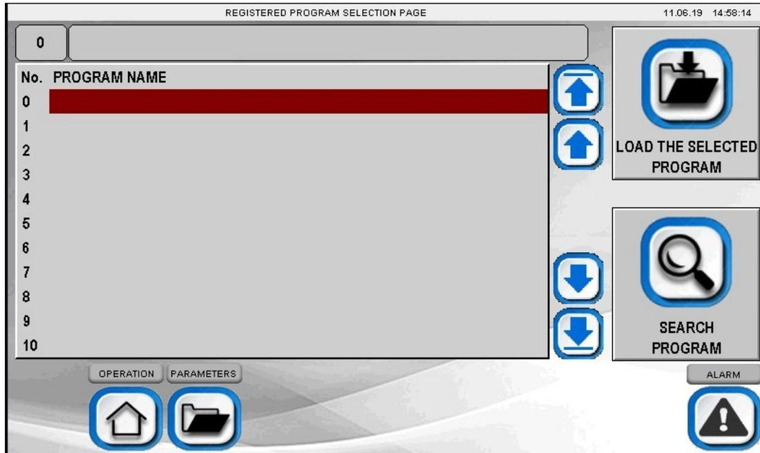
**Load the Selected Program:** To load welding and annealing properties that for selected saw properties which is set and saved before. When the user chooses a program and click 'LOAD THE SELECTED PROGRAM' button, assigned Welding & Annealing settings are set automatically and machine is ready to welding & annealing processes. The machine waits the user to pressing START button.
