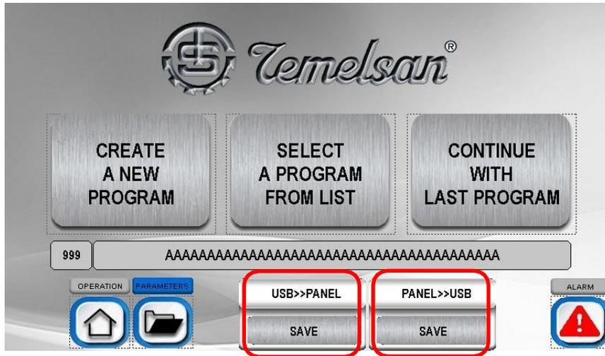
**USB >> PANEL SAVE:** This option helps to you Welding & Annealing settings transfer from USB Memory Stick to the Machine.(For this operation Barcode reader USB input could use.)
