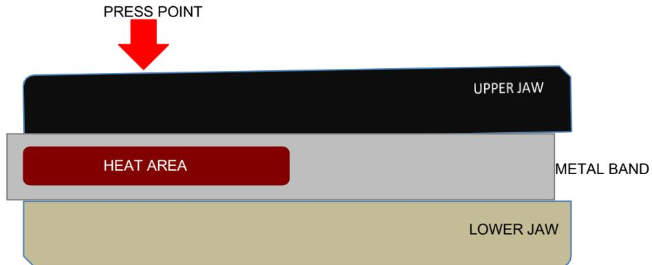
To keep similar Annealing clamping Press Point on both Clamping Jaws it's always recommended independently how tight the screws are turn able to work with an Allen key and using it as an dial like on a watch or dial indicator, in 5 minutes steps or 10 degree.
