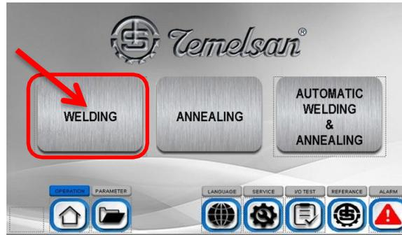
This process provides the desired welding with the parameters to be entered manually. The options below appear on the screen when user click Welding button.
