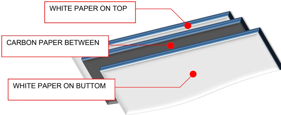
The Carbon Paper Print is showing similar print picture on both clamping jaws as an perfect similar adjustment.
