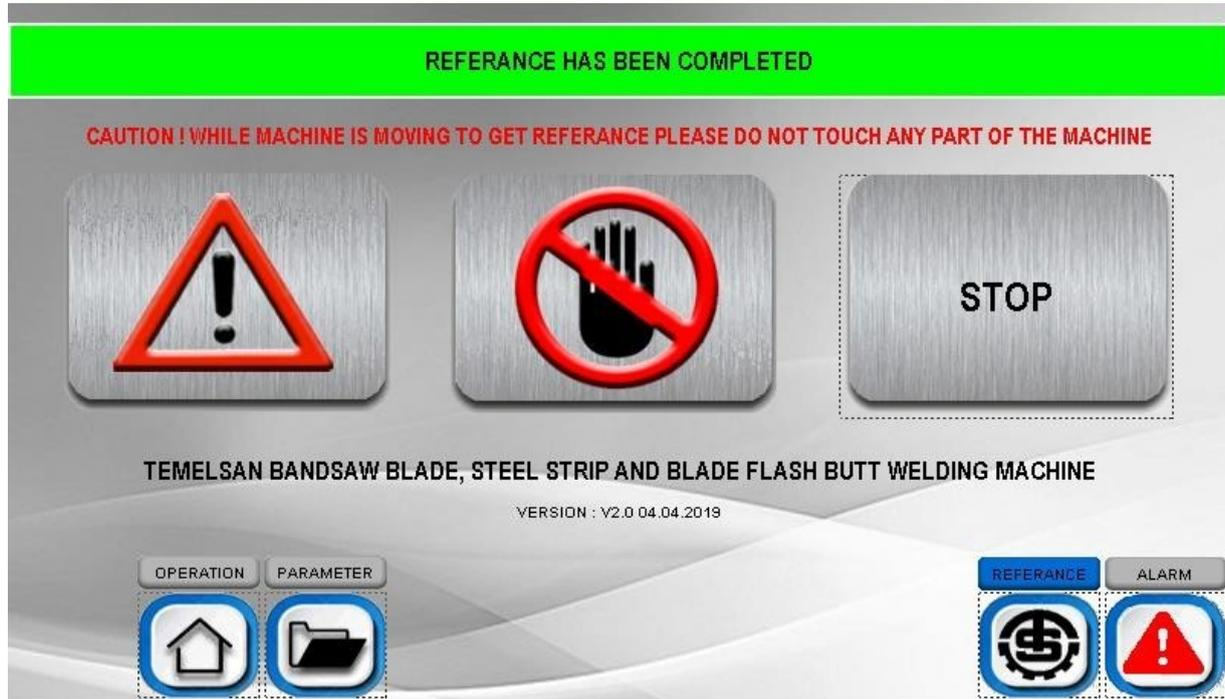
Green colored box with 'REFERANCE HAS BEEN COMPLETED' text indicates the reference is completed and the machine is ready to use.
