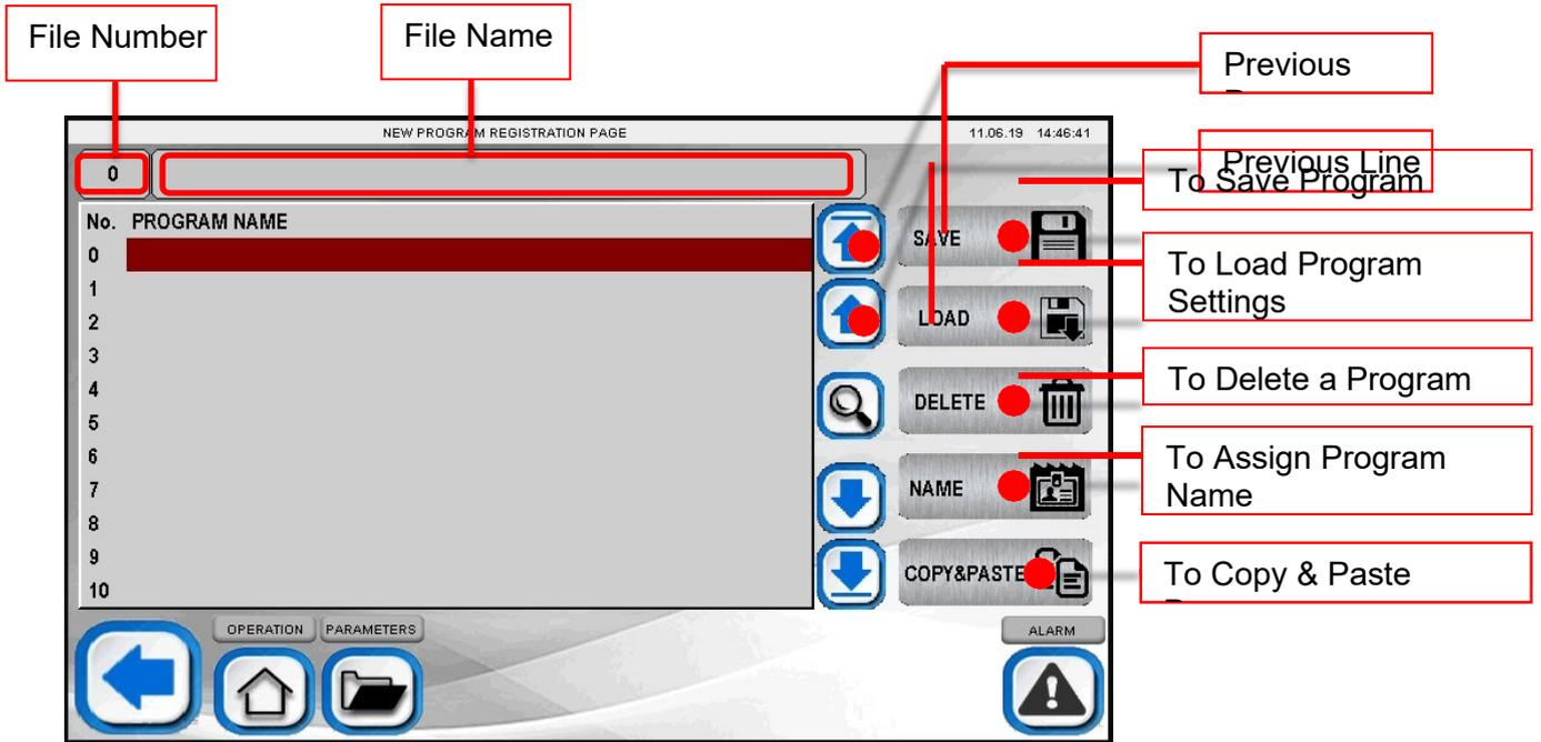
When user touched on the program name section a Keypad appears and the user could give desired name of your setting easily. Also the user can save the program to particular file number by clicking on the number which user wants to save.
