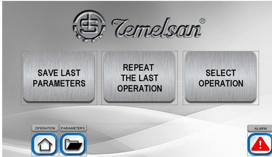
**Save Last Parameters:** Saves the last parameters which have been assigned settings on last welding. If welding quality is satisfying, the user can save welding parameters by this button.
