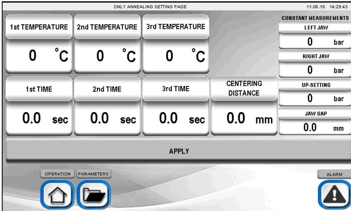
**1<sup>st</sup> Temperature:** Temperature value that to be reach of first step of annealing.
