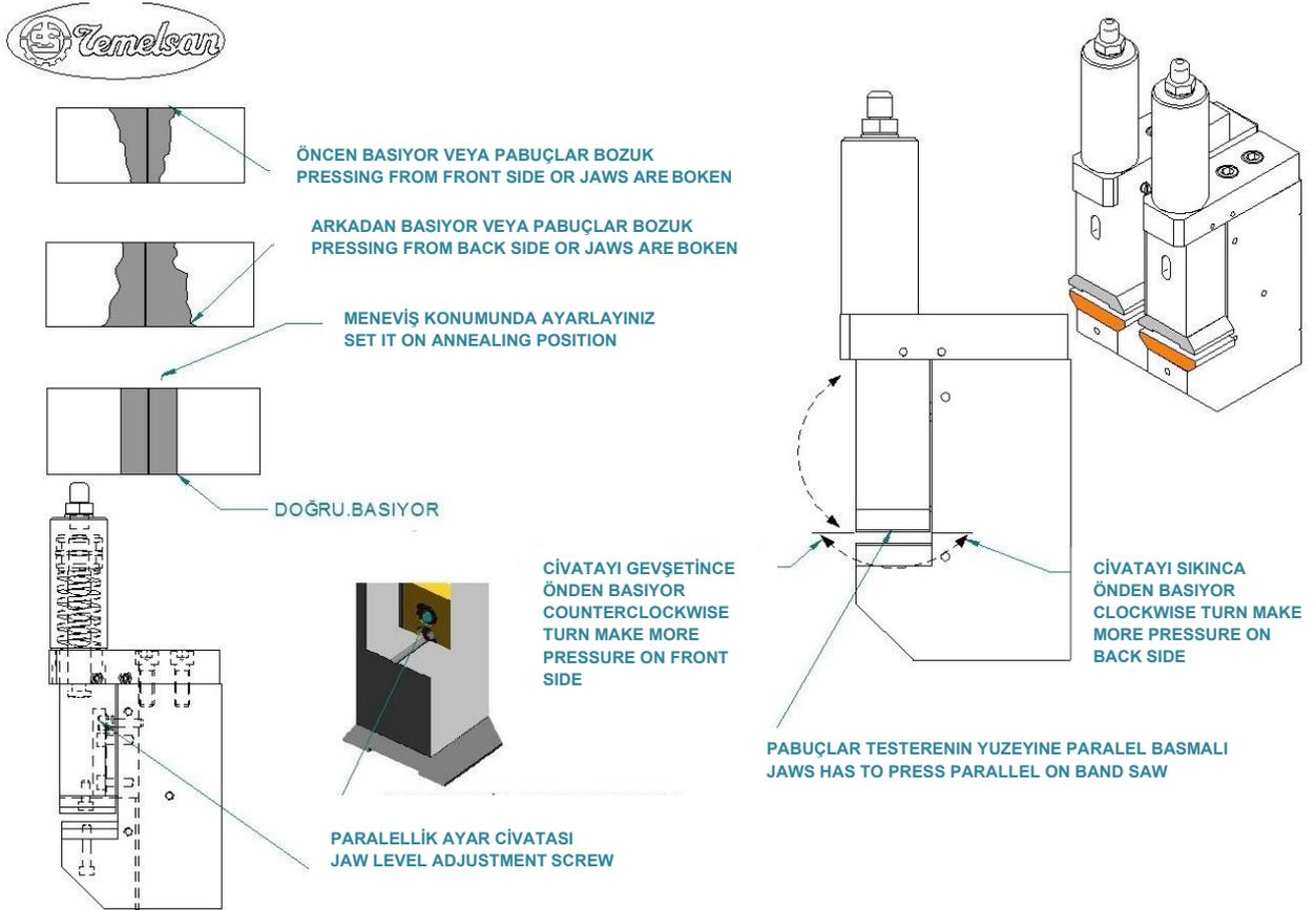
Turn the Jaw Level Adjustment Screw clock wise (to the right side) the Upper Jaw will create more clamping pressure on the front side. Turn the Jaw Level Adjustment Screw opposite direction (to the left side) the back clamping pressure between jaws will increase.
