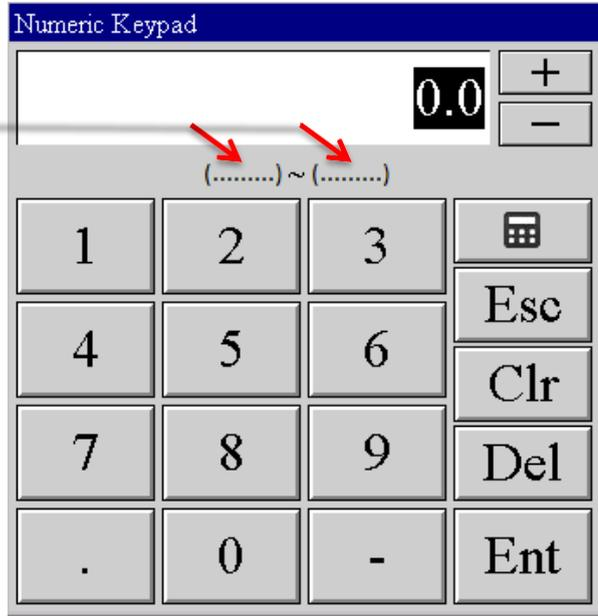
**Welding Current:** To set welding current as percentage. (0 - 99%) (\*Note: Welding Current is one of important setting for qualified welding.)
