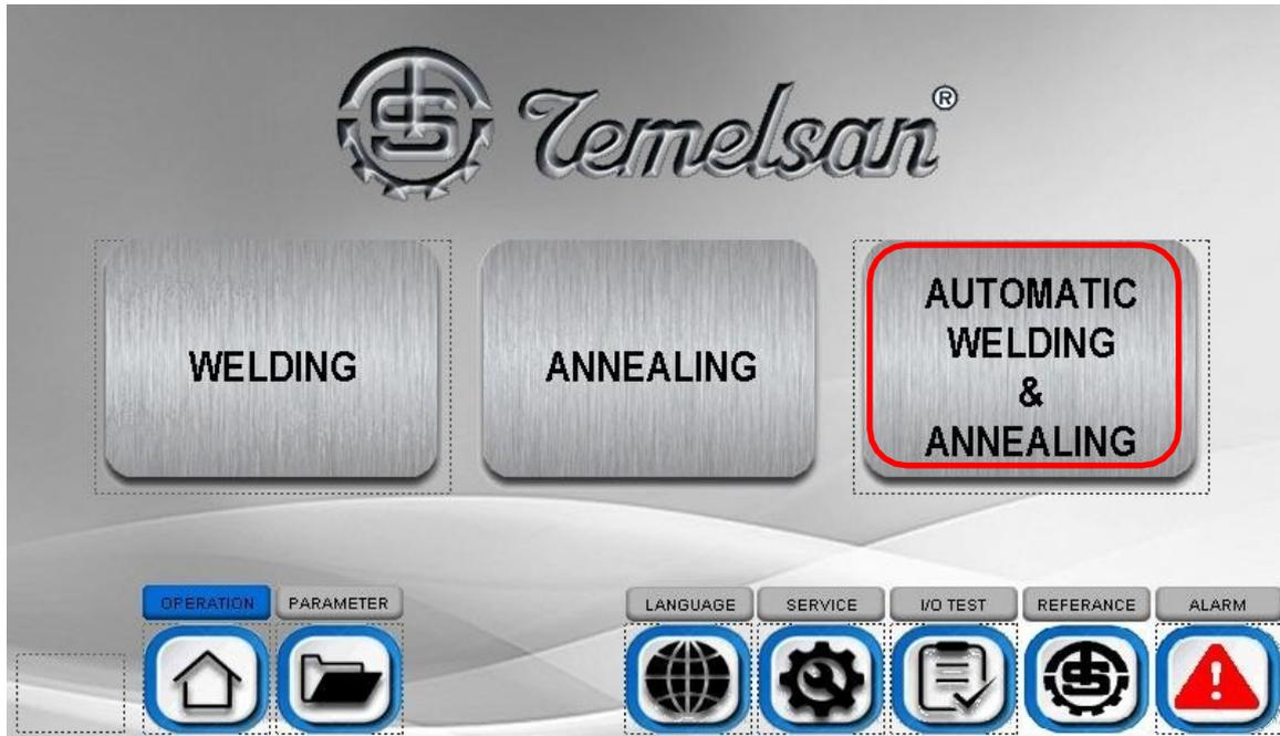
This process provides the desired welding and annealing with the parameters to be automatically. The options screen at below shown on the screen when the user clicks on Automatic Welding & Annealing button.
