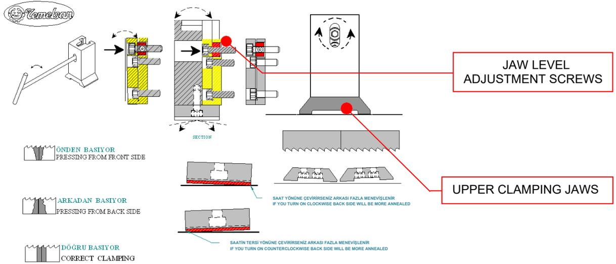
With changing of Annealing Press Point we are able to clamp properly all different width of Metal-Band
