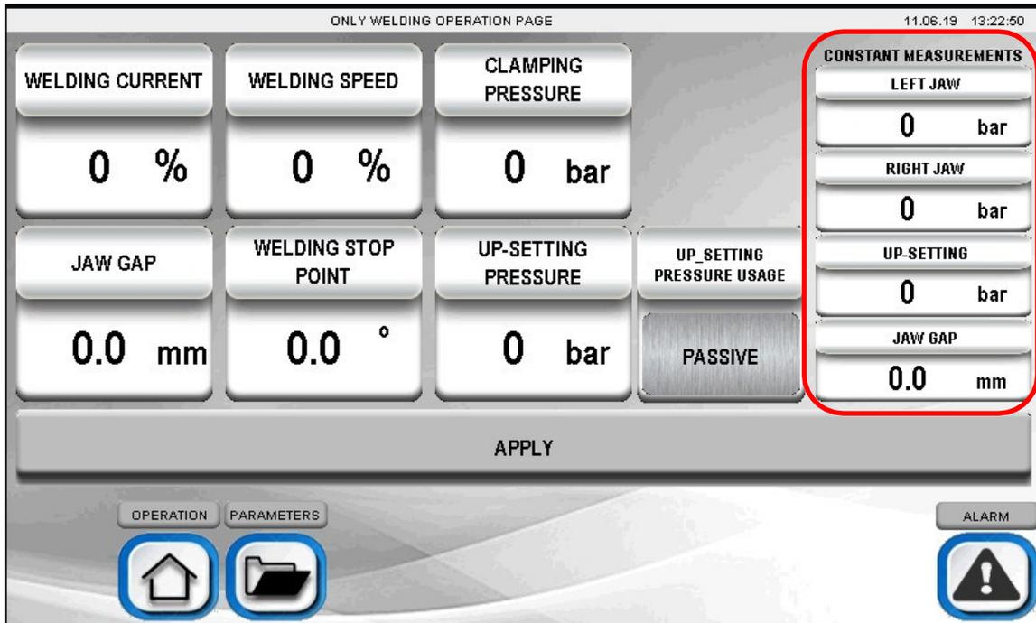
The right side of the screen shows the instantaneous values of Left Jaw Pressure, Right Jaw Pressure, Up-Set Pressure and Jaw Gap Distance.
