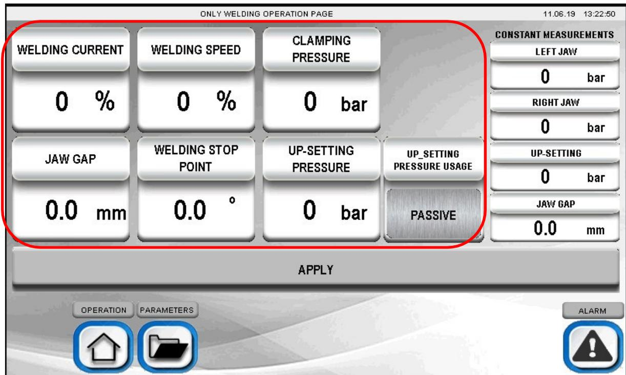
The user can assign the value which want to change by simply clicking on it. When the user click on it, a numeric keypad appears shown like at below.
