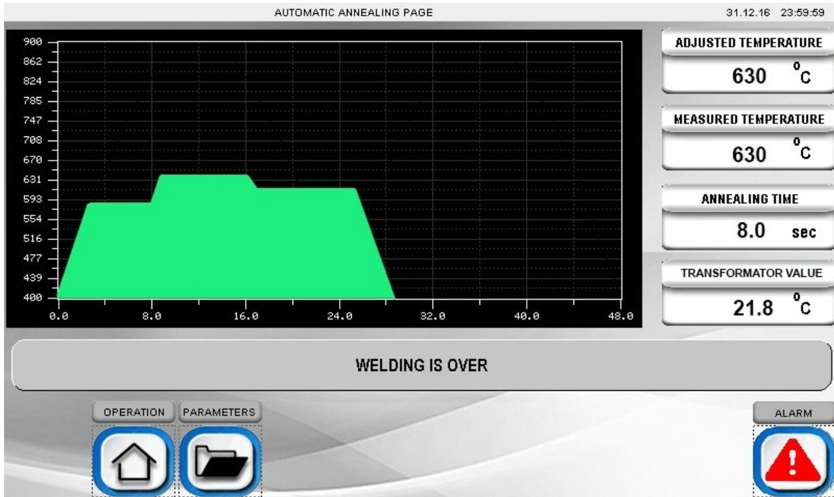
Additionally, the annealing times starts at the degree which given by the operator. Before the annealing process the material is heated and after annealing process the material is cooled under control by the PLC. The descriptions of time intervals are shown below at the graph.
